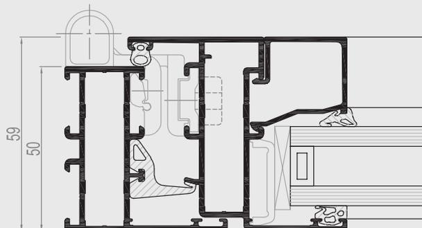
CS 59Pa offers an extensive range of non-insulated profiles for the construction of elegant and moderately priced aluminium frames in functional style. Therefore CS 59Pa is the ideal system for outdoor applications in warm climates but it can also be used for the partitioning of indoor office spaces.
